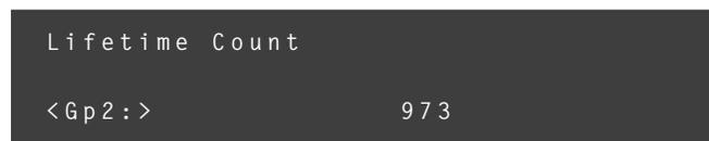
4. Scroll to see the number of times the Hot Water Tap button has been engaged
